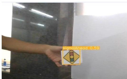
Fig. 12: Detection of signal ahead road sign
