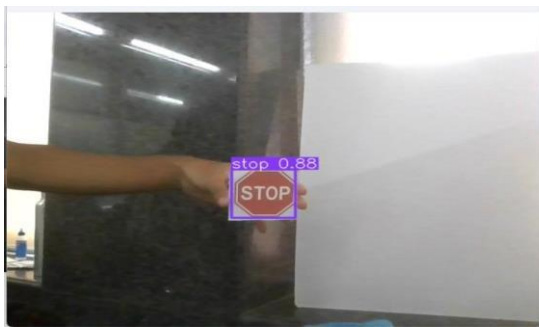
Fig. 11: Detection of stop road sign
